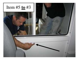
Loosely bolt **Center Divider** to **Front Bulkhead**
